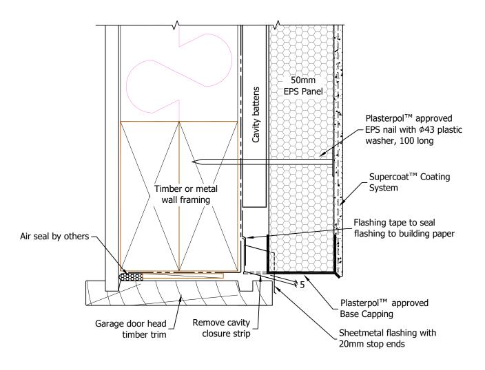
NOTE Above detail is only suitable for standard roller or sectional roller garage doors
